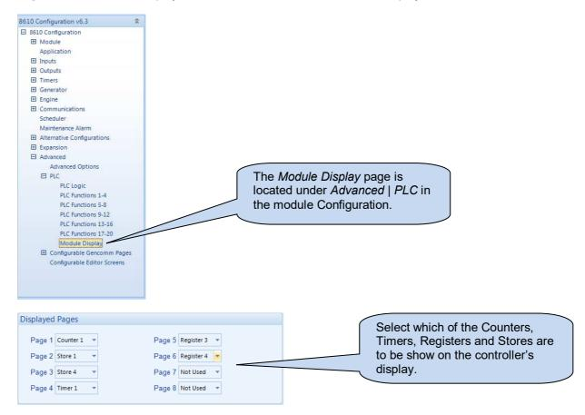
After selection for display on the host controller, *Counters, Timers, Registers* and *Stores* are able to be viewed and/or edited as below on the controller display.
