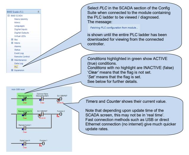
Example showing SCADA display of Flag Testing:
