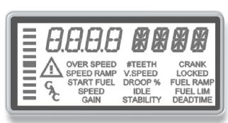
The EEG6500 Series Quikset Display allows its operator to monitor and configure parameters without any external monitoring devices. This means no configuration software or PC required.
